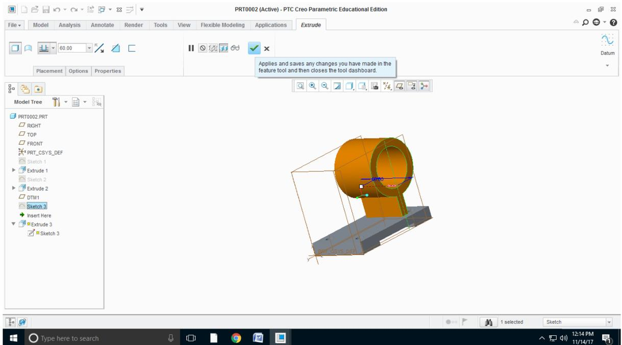
Step 10: Create an datum plane at specified distance and select Rib Command from Model
