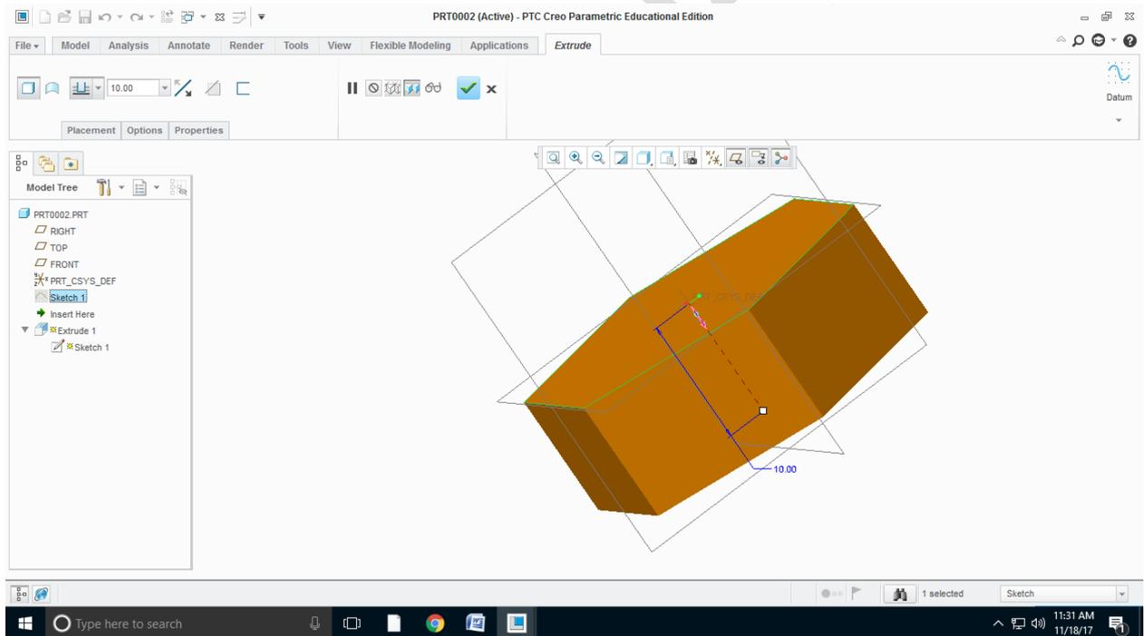
Step13:Select a datum plane as shown in figure and with reference to that draw the required shape to smooth the bolt surface using revolve option nad save it
