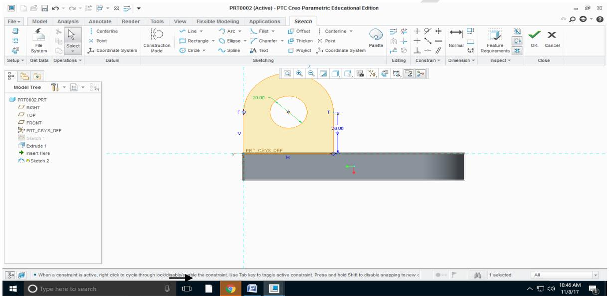
Step8: Extrude the sketch and specify the width and direction of extrusion Click on ok
