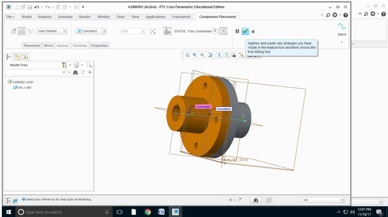
Step 20: similarly do the assembling of remaining parts to get complete of the flange coupling assembly
