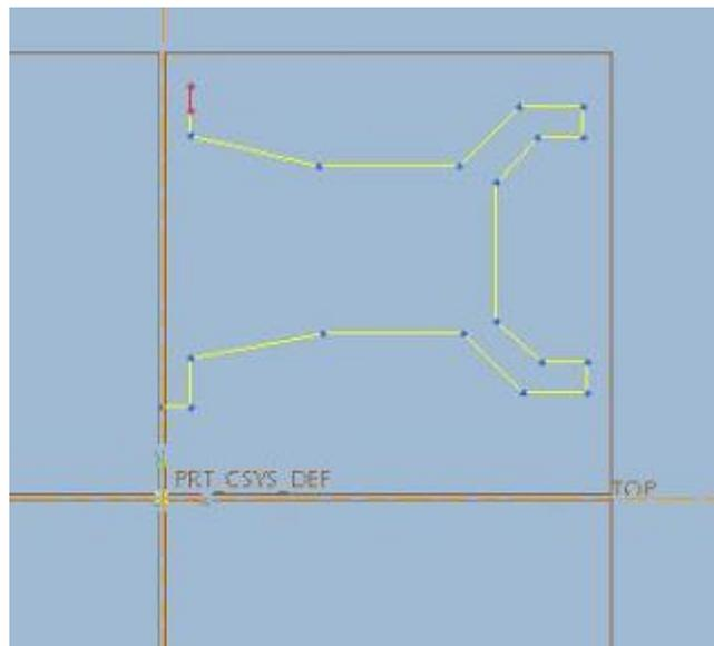
*Fig: Sketch of piston to be revolve*
