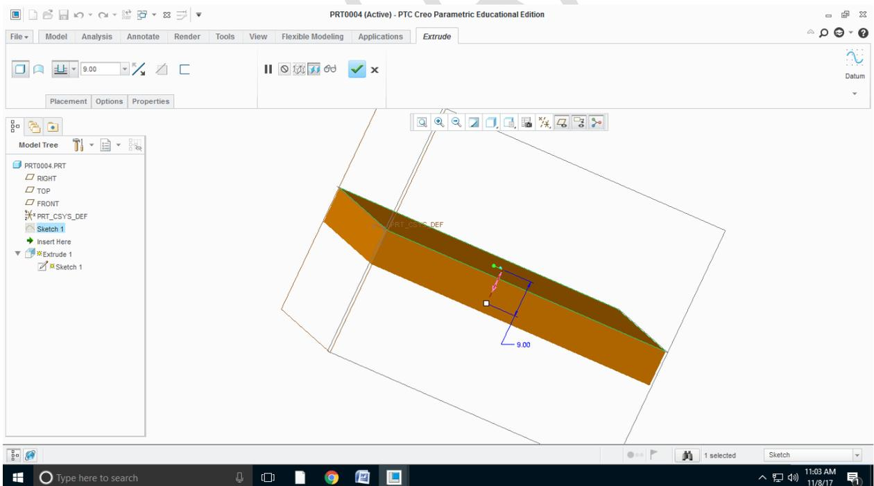
Step7: select the required surface to add the material of the part and also draw the required sketch.
