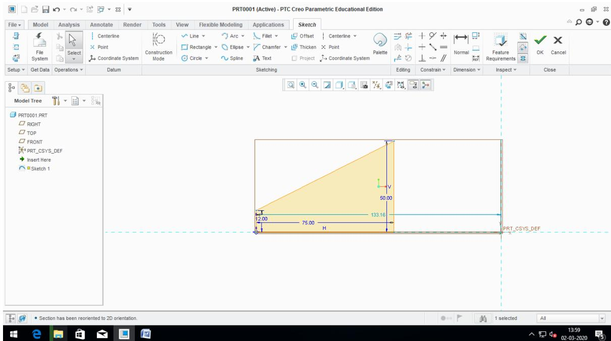
Step6: Extrude the sketch perpendicular to sketch plane. and Specify width and direction of an Extrusion and Click on ok
