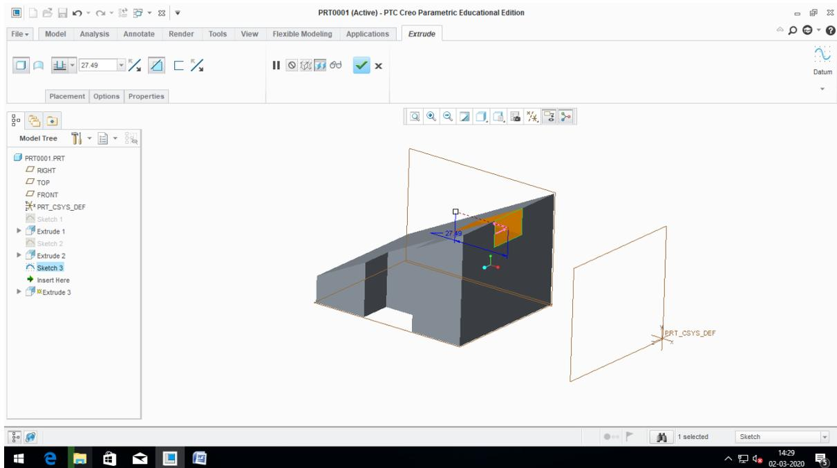
Step8: Extrude the sketch by using Symmetry option and specify the width and direction of extrusion and Click on ok
