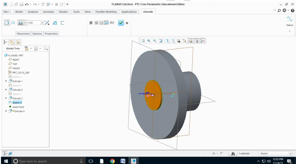
Step9:select the required surface to remove the material in the hub and then draw the shaft in 2d sketch plane and extrude it by giving the required dimensions
