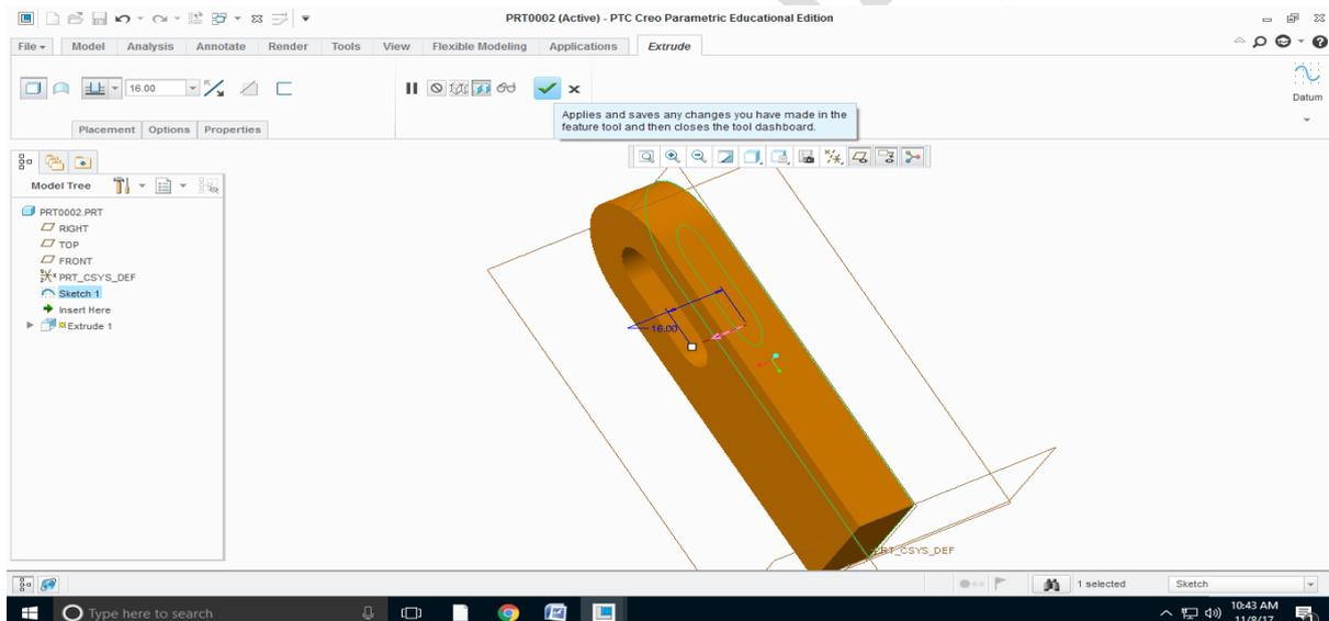
Step7: Select Extrude → Required surface → Sketch View option → Specify references → Draw the required sketch as shown in **Figure.2** Click on ok
