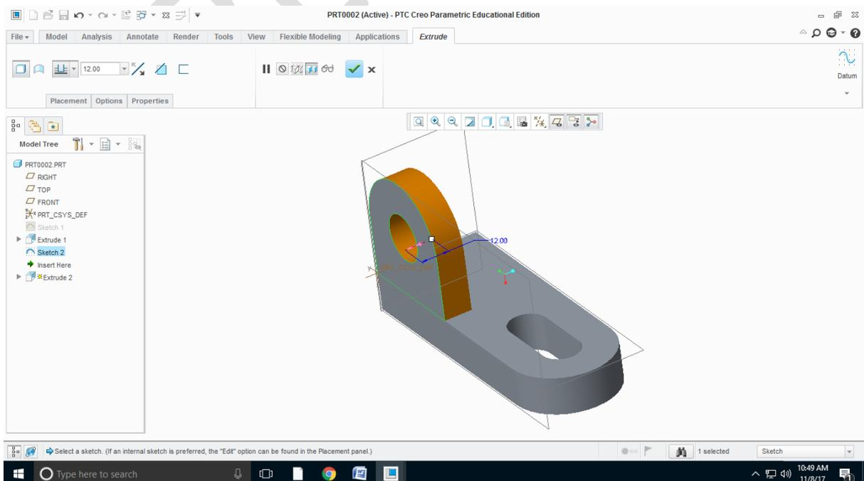
Step9: Select the datum plane at the middle of the sketch and select the part which is to be duplicated then select the mirror and then select the plane to complete the object Click on ok
