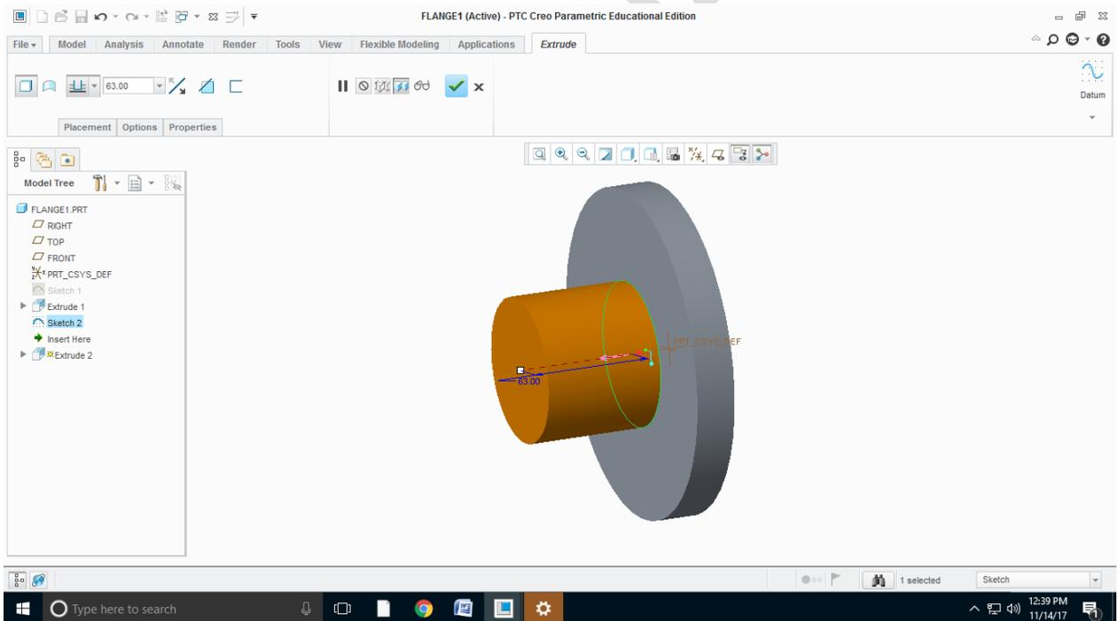
Step 8: select the required surface to add the material and then draw the hub in 2d sketch plane and extrude it by giving the required dimensions
