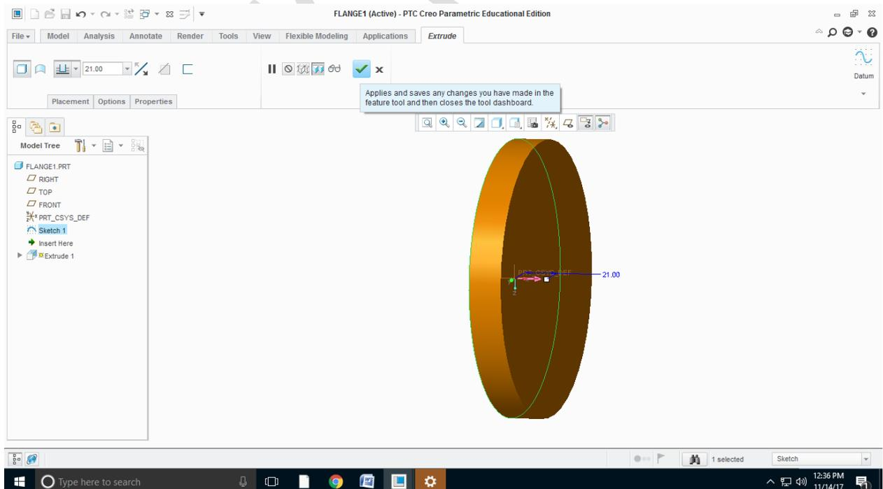
Step7: select the required surface to add the hub and then draw the hub in 2d sketch plane and extrude it by giving the required dimensions
