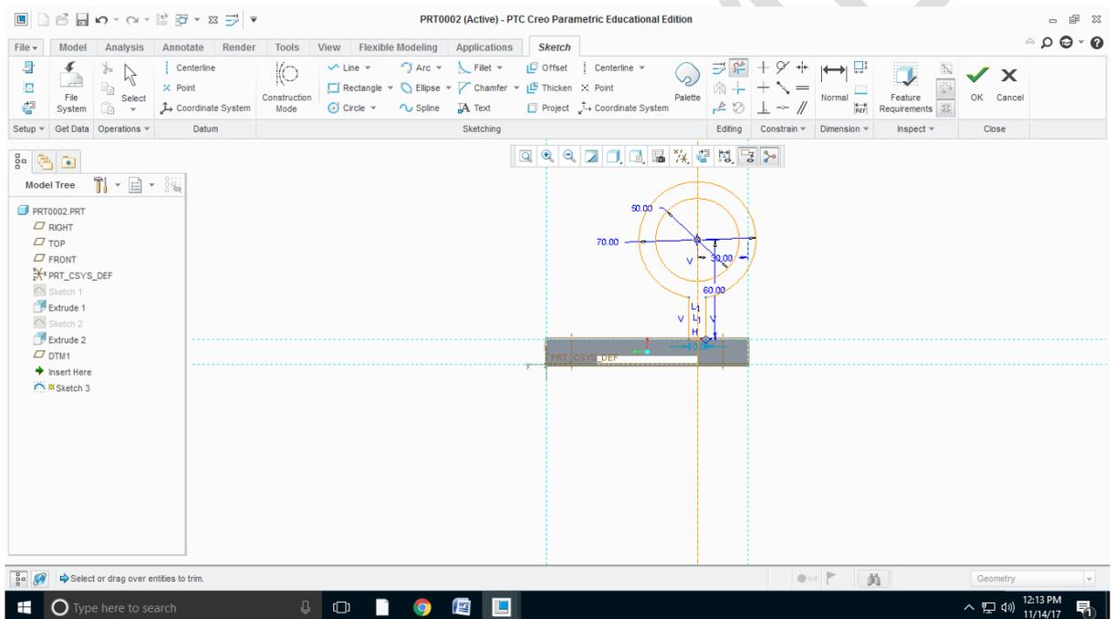
Step9: Extrude the sketch by using Symmetry option and specify the width and direction of extrusion and Click on ok
