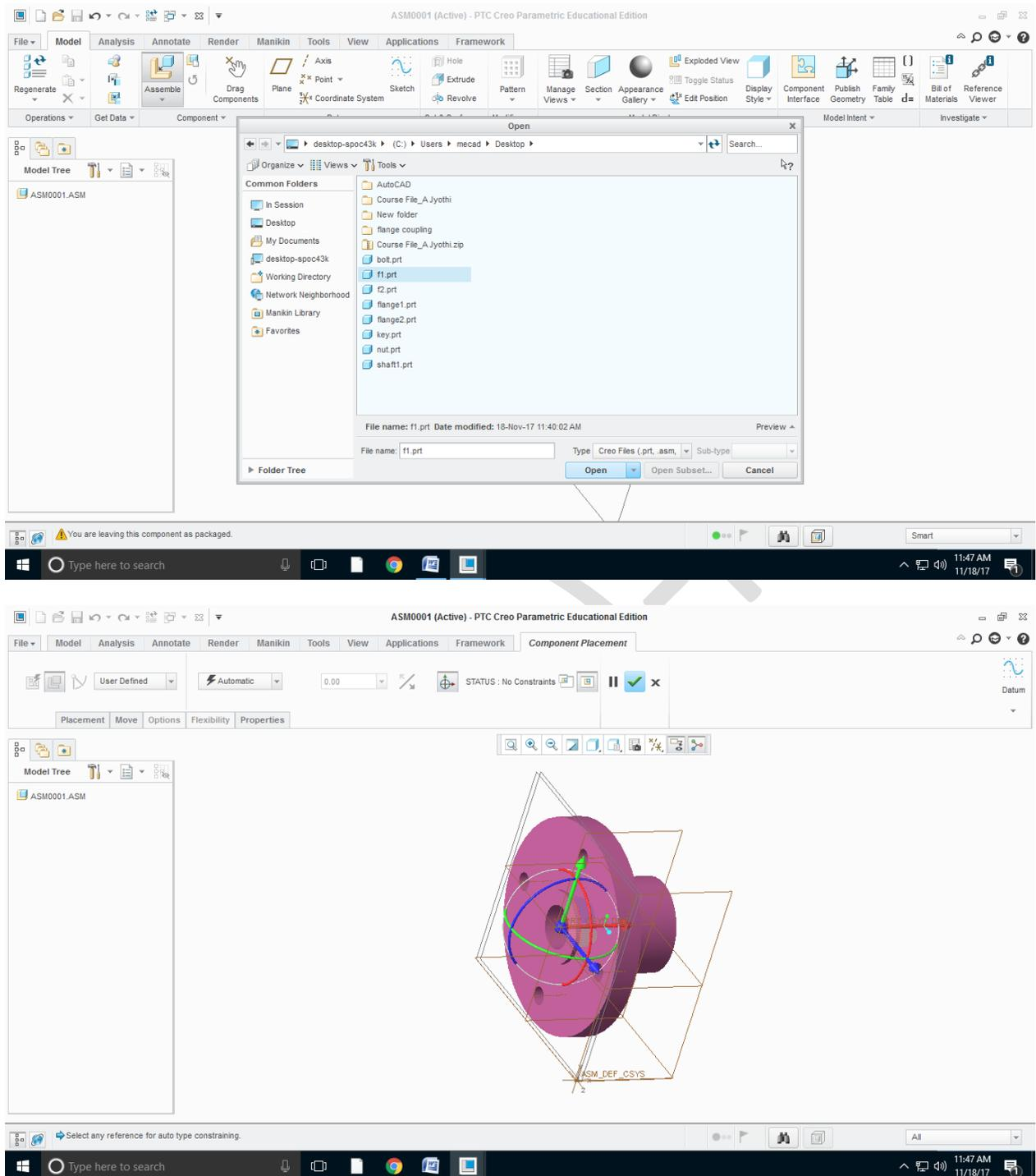
Step 19: Similarly get the 2<sup>nd</sup> part to do the assembling and select the coincide option and select the parts and axis to be coincided.
