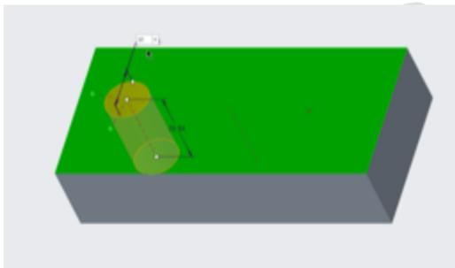
Step8: Create the datum plane at the distance 40 mm from one end of the surface along the length of the sketch and with this as a reference plane draw the required shape of the object and Click on ok
