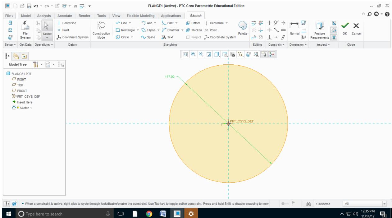
Step6: extrude the sketch perpendicular to the sketch plane and specify width and direction of extrusion
