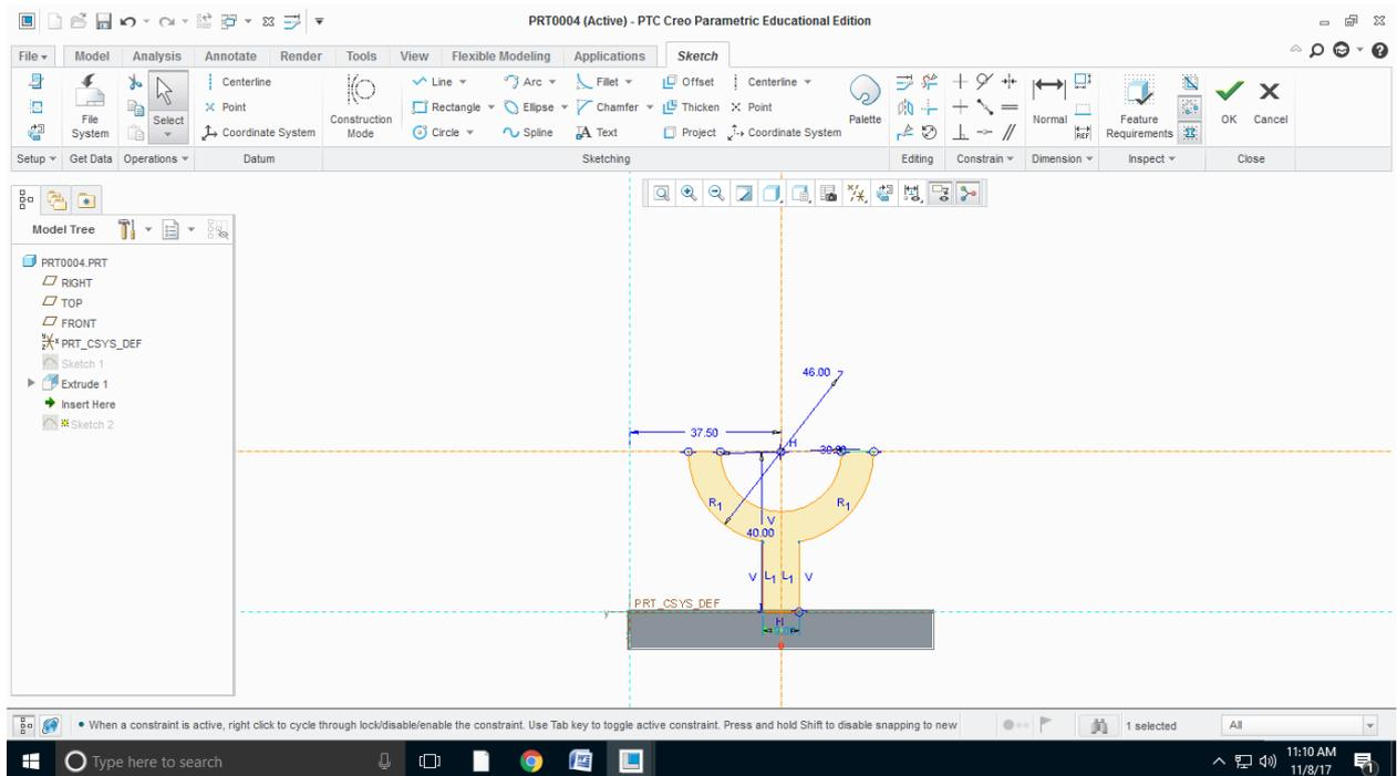
Step8: extrude the sketch and specify the width and direction of extrusion
