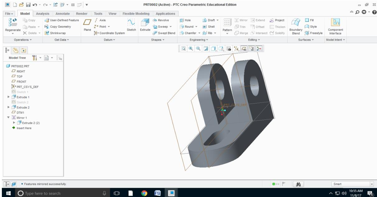
Step10: Round the edges of a part to a specified radius by using Round Command Click on ok
