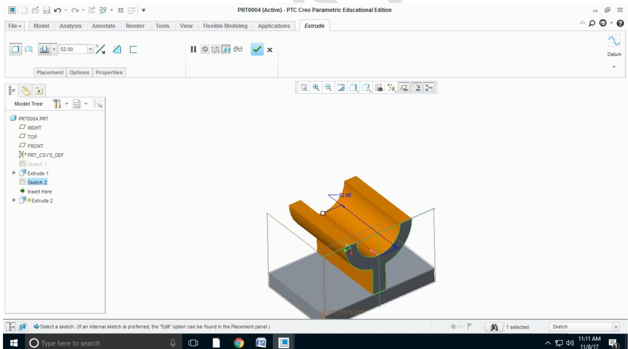
Step9: select the datum plane at the middle of the sketch and with reference to that plane draw the required shape of the object and then extrude it with require dimensions.
